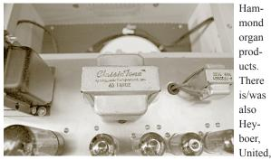
and Magnetic Components. There is typically an EIA code as the prefix to the date code just like on speakers and pots.
